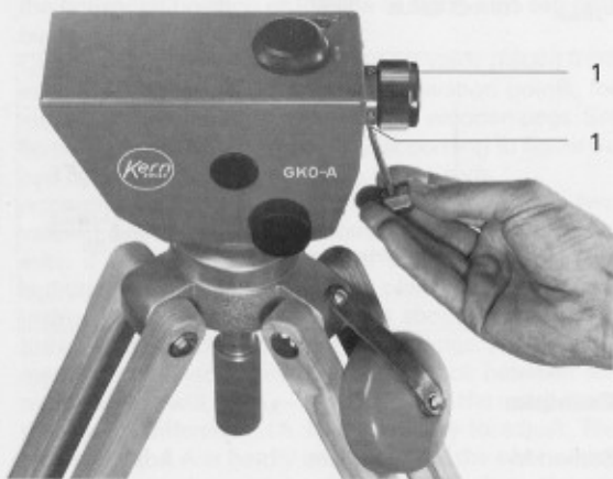
Fig. 7 Adjustment of the line of sight 1 Adjusting screws
